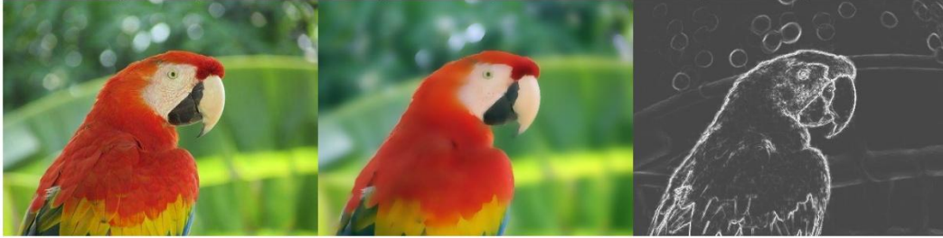
Image Segmentation with Ambrosio-Tortorelli approximation of Mumford-Shah functional original image segmented image regularized edge set
